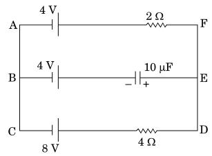
In the given circuit, with steady current, calculate the potential drop across the capacitor and the charge stored in it.
